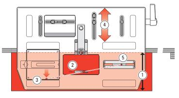
**6-22 Mortises in center of boards 45/8" to 6½" [115 to 165mm]** ①: Mark mortise center on a test board ②. Using the guide recess front edge as mortise guide ③, adjust the table to center the mortise ④. Control mortise length with  $\frac{3}{16}$ "[5mm] dowel pieces in the pin track ⑤ (see 6-16). *Note: This is not a standard Leigh solution, but we thought it would solve this rare challenge.*
