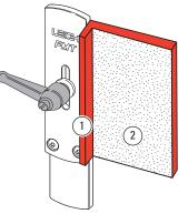
**6-4** This packing piece should include its own side-stop fence ① and if required frequently, should have sandpaper glued onto its outer surface for secure workpiece clamping ②.
