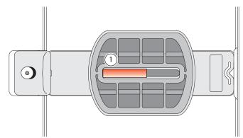
**6-16 Mortises** The rule is the same for mortises except you will need to use a small piece of that  $\frac{3}{16}$ "[5mm] dowel as a guard in the guide's mortise slot ①. The dowel should be slightly longer than the difference between the guide length and joint length; in this example, slightly longer than 1"[25mm]. In this example, the joint is only 1" long and the guide mortise slot is 2". So you need a guard dowel to prevent cutting a mortise longer than required.
