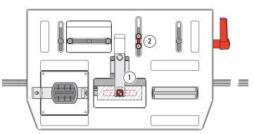
**6-6 Tenons** Mark the center as before. Position and sight the tenon ①, and lock the table. Set the **βFB** stops against the post ②.
