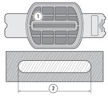
**6-5** The FMT Pro table movement allows for easy routing of oddsized joints. For example, you may want to rout a 3"[75mm] joint ② and you only have a 2"[50mm] guide ①. Use this simple formula: Joint, minus Guide, divided by 2.
