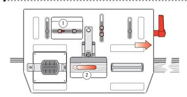
**6-11** Move the table **right** to the stop ①. Rout the **right-hand** end of the mortise ②, using the full length of the mortise guide.
