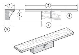
**6-19** Make this bracket to mount and mortise a wide board face, clamp pieces greater than Leigh Clamp 3" capacity, and center mortises on boards up to 45%"[115mm] wide or even 63%"[162mm].
