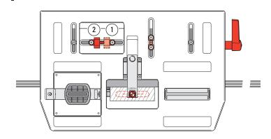
**6-7** Set the **abulk** stops one at a time with the small block between the stops and post ①②. This ensures that the table movement is centered about the joint center-mark on the stock. Remove the block, **but save it**.
