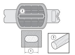
**6-13** For mortises and tenons shorter than the guide, reverse the calculation: Guide, minus Joint, divided by 2.
