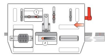
**6-12** Move the table left to its stop ①. Rout the left-hand end of the mortise ②. Repeat for all required mortises. So to recap; for joints longer than the guides:
