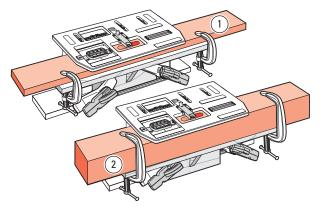
**6-21** Use C-clamps to hold the workpiece onto the bracket, with the workpiece rear edge touching the clamp plate. Now raise the bracket so the workpiece touches the underside of the table. Re-secure with the Leigh Clamps. The widest board in which a mortise may be centered is 4½"[115mm] ①.The thickest capacity is 4"[100mm] ②.
