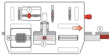
**6-10 Mortises** Release the table clamp. Use the small block between one stop and the stop post ① and lock the table clamp. Center a mortise piece under the sight and clamp ②. Set side-stop blocks or marks on the outriggers ③.
