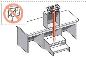
**6-18** To rout long vertical boards you could build a jig stand to mount on your bench. Make the stand/bench combination high enough to accept the desired board length. *Bolt securely to the bench*. Make a stable platform as shown here to stand on. **Don't use a folding step, these are unstable.** Other novel solutions: holes in (suspended) floor; jig bolted to deck or mezzanine railing; wall brackets.
