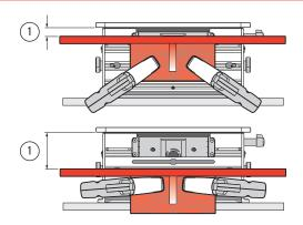
**6-20** Use the Leigh clamps to secure the bracket to the FMT Pro clamp face and adjust the distance below the table to slightly greater than the mortise piece thickness ①.
