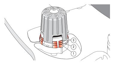
**4-10** Check that the left hand knob is two turns up. From this setting the actual fit setting will be established by trial and error and the result recorded for each guide/bit combination. Note: The "steps" in the height "washer" indicate numbers of "turns up"; one turn ① two turns ② three turns ③ Never turn the knobs up more than  $3\frac{1}{2}$  turns in use.
