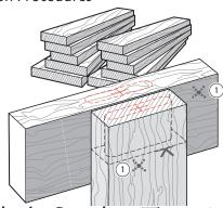
**4-27 Production Procedures** When routing frame joints it is only necessary to mark and sight a single tenon and perhaps two mortises. Once the side stop fence or outriggers are set and the table sighted for one joint, any number of similar joints may be routed without marking and without removing the router from the jig. We recommend marking the finished face which goes against the clamp plate (shown here from operator view) ①.
