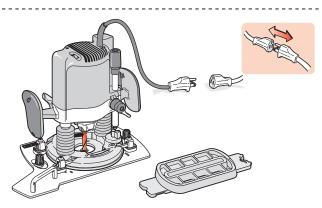
**4-7** Unplug the router. Insert the selected guide in the guide recess and the matching diameter bit to the router. Note: See Appendix I for Guide and Bit Selection.
