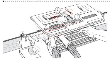
**4-29 Mortises:** Sight one mortise ① and set a stop block at the end of the mortise board ②. Set ap LR limit stops and &FB limit stops to prevent unintentional table movement 3.
