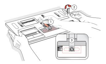
**4-3** If you have not yet mounted the side stop fence, do so now (see 3-13 to 3-15). Place it off center by about half the width of the tenon piece; either side, it doesn't matter. Pull the table sight forward to its stop ①. Release the table clamp ② and move the table to position the sight over the approximate tenon piece position ③. Lock the table. Always lock the table before positioning workpieces.
