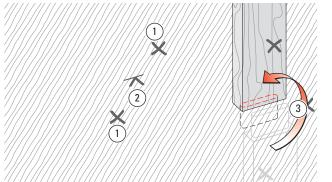
**4-2** In almost all cases, it is critical to have the same side of workpieces reference against the clamp plate for each tenon and mortise. Mark one side of each workpiece to reference "this side toward the clamp plate" ①, or "away from". Make a pencil mark ② to the required shoulder depth on the tenon workpiece. When the joint is cut, the tenon piece is rotated 180° to assemble ③.
