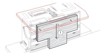
**4-39** For very small joints we recommend attaching a rigid piece of ply or MDF minimum 3/4" [20mm] to the clamp plate, using the through screw holes in the plate. This should have its own mini side stop fence attached for tenons ①.
