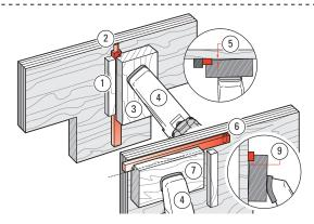
**4-40** To hold very small workpieces ②, make up a rabbeted holder 3 with the rabbet slightly shallower than the workpiece thickness, leaving a gap at ⑤ and ⑨. i.e. For Tenons: Side stop ① Tenon Piece 2 Holder 3 Clamp 4 Gap 5. For Mortises: Mortise Piece ⑥, Holder ⑦, Clamp ④, Gap ⑨. ■
