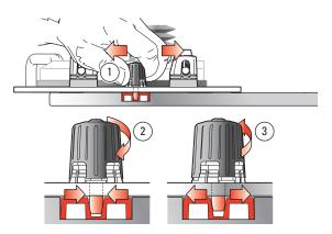
**4-9** Adjust the right hand guide pin. Grip right hand pin knob and move sub-base back and forth to feel the "free play" of the pin across the slot width ①. Turn knob down 1/8 of a turn at a time, to feel the "play" diminish ②. When the "play" stops, turn knob up 1/8 of a turn until the slightest play can be felt ③. The router/sub-base should slide freely left to right. If right pin is a little "sticky", turn it up a bit more.
