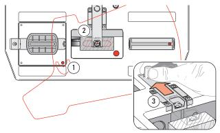
**4-28 Tenons** The router is "parked" with the guide pin in near front corner of recess ①. Extend sight and use only as a tenon stop ② when clamping successive (unmarked) tenon pieces against side stop. Retract sight 3 and rout any number of tenons without removing router. Note: If you forget to retract the sight, the Sub-Base will push it out of the way as you move it rearward, but we do not recommend this.
