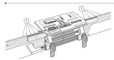
**4-31** Successive mortises in "ladder" type construction are quick to rout. Mark all mortises on only one piece (only one needs a front-toback mark!). Sight the first mortise (cross) to set the table and mark the top of one outrigger in line with the workpiece end. Table locked, move the workpiece, sighting each successive mortise line, marking the outrigger(s). To rout, align the unmarked board ends with the outrigger marks 1.
