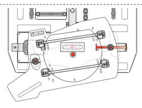
**4-8** Make sure the two guide pins are turned up two full turns from the lowest position!
