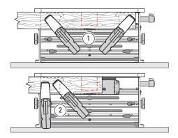
**4-15** Remove the router and tenon workpiece from the jig. Position the two clamps so the mortise piece can be positioned for secure holding. Clamp to either both sides of the vacuum box ① or to one side ②. Note: Leaving a "horn" on the ends of mortise pieces as in ① not only makes for easy clamping, it's good woodworking practice as the horns will be an aid in assembly gluing and clamping later.
