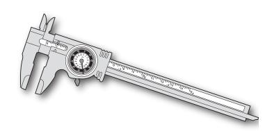
**4-24** If you have a dial or digital calliper (every shop should have one) you can literally measure the tenon and mortise and adjust accordingly.
