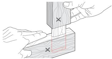
**4-20** Remove the mortise piece and test the tenon for fit and (keeping the marked faces adjacent) for flushness. If the face sides are not flush, check the straightness of the two parts. If they are straight, the clamp plate may not be vertically parallel to the bit. See Appendix II, Jig Adjustments, A2-1 through A2-3.
