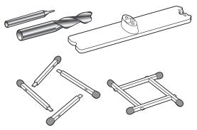
**4-38** The tiny  $\frac{1}{32}$ " x  $\frac{3}{32}$ " [0,8 x 2,4mm] mortises and tenons on this "match frame" were formed (with machine tool bits) on a 1/4"x 5/16" guide. The 15/32" tenon bit is 7/32" larger than 1/4". The 1/32" bit is 7/32" smaller than 1/4". A similar metric set: 6mm guide; 1mm mortise bit, and 11mm tenon bit to produce 1mm joints. Machine tool bits as small as 0.010" with 1/4" shanks and similar metric are available from machine tool suppliers.
