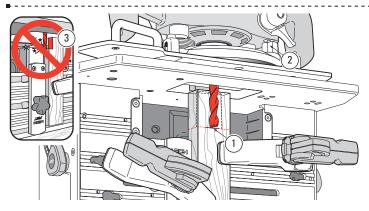
**4-11** Plunge the router so the tip of the bit is level with the pencil mark of the tenon shoulder and lock the plunge ①. Set the plunge depth stop rod to its stop ②. *Generally, tenons are routed in one depth setting, it is not necessary to make multiple passes at different depths of cut.* WARNING: Never rout tenons with the sidestop fence in the inverted position ③.
