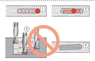
**4-18** The best way to rout mortises (parallel to workpiece) is plunge full depth, slightly overlapping holes ①, then clean out left-right-left at full depth of cut 2. Do not rout left-right-left at progressively greater depths without plunging holes 3 ... the bit's rotation will pull the bit off the intended mortise line with each pass 4 and the mortise may not be parallel to the workpiece.
