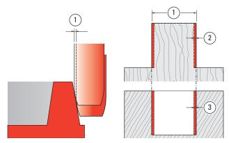
**4-22** How much adjustment is required? One eighth of a turn of the guidepin knob will change the joint glue-line fit by 0.001"[0,025mm] ①, i.e. turn one-eighth up; the bit will reduce the tenon thickness by 0.001"[0,025mm] (half of that **per side** ②) and increase the mortise width by the same amount ③. Dimensions and angles shown here are exaggerated.
