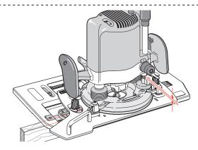
Place the router/Sub-Base assembly on the jig, the left hand guide pin in the mortise slot part of the guide. Now raise the plunge stop rod slightly, say 1/32-1/16" [1-1,5mm] to allow the mortise to be routed slightly deeper than the tenon to ensure perfect tenon shoulder flushness on the finished joint.
