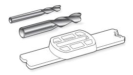
**4-33 Two Bit Combination** If you want to rout many ¼"[6mm] mortises and tenons, the tenons can be routed much more quickly with a ½"[12mm] bit\*. The Guide and Bit Selection charts in Appendix I show how different bit combinations can crank out such extraordinary joints just as quickly and precisely as larger ones, and with adjustable joint tightness.
