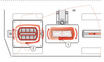
**4-12 Read all of the next 3 instructions before routing.** With guide pin in near side of guide recess, switch on router power and with firm control, move it in until the bit lightly touches the tenon workpiece. Very carefully, with bit very lightly engaging the wood surface, "climb rout" clockwise around tenon piece ①. Maintain very light bit contact. Do not run guide pin on guide yet ②.
