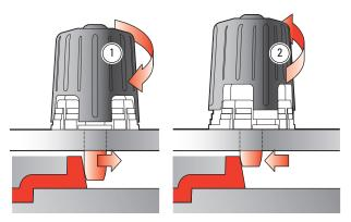
**4-21** If the joint is too loose, turn the LEFT guide pin down ①. If it's too tight, turn the LEFT guide pin up ②. For how much, see 4-22. Rout a complete new joint. *Note: It's possible to adjust the guide pin and rout only one new mortise or tenon part and get a good fit, but on a project this would mean routing each part at different settings. Establish ideal pin height for both mortise and tenon at one pin setting.*
