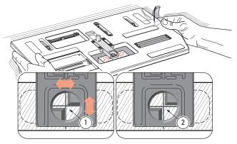
**4-5** Release the table clamp and move the table until the sight opening is positioned equally around the cross lines on the workpiece. Lock the table. Because the human eye excels at comparisons, differences as small as 0.004" can be perceived in the space between the edges of the line and the triangles as shown here ①. You can readily center the sight using slight table movements until the spaces appear the same ②.
