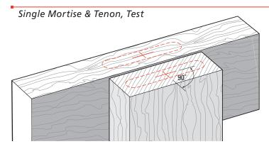
**4-1** Let's make a plain single mortise and tenon. Using a fine pencil, mark a cross at the center of the required tenon and mortise. The cross lines along and across the axis lines of the joint must be at 90° to each other. Mark the mortise several inches[10cm] or so away from the end.
