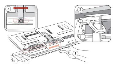
**4-16** Extend the sight. With the marked side of the mortise piece toward the clamp plate, either move the board left and right 1) to align the cross with the sight and clamp in place; or clamp in place first and move the table to align the sight 2. Remember, you previously set the **FB** limit stops to allow only left/right movement. For routing very small pieces ③, see 3-16.
