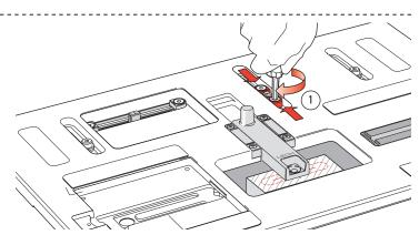
**4-6** Unlock the two **9 FB** front/back limit stops. Move both so they touch the Stop Post and tighten both stops ①. This prevents front-to-back movement of the table when later sighting the mortise. Retract the sight.
