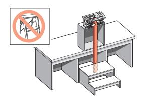
**1-3** For routing long vertical rails it may be necessary to build a jig stand to mount securely on your bench. Make the stand and bench height combination sufficient to accept the board length you have in mind. *The jig stand should be bolted securely to the bench.* Make up a stable platform as shown here to stand on. **Do not use** a collapsible step stool, these are unstable and unsafe.
