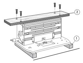
**1-2** Turn the jig upside down on two wooden blocks ① (to protect the table and sight knob). Using the four nuts and four flathead countersunk machine screws, bolt the base board to the jig using the two nut recesses in each end housings. The ½"[13mm] front edge ② to the front of the jig (of course). Now you can clamp your FMT Pro to any bench.
