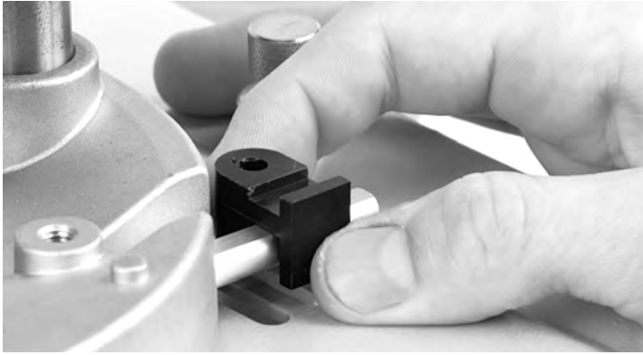
2-3 Take the rod clamps and by trial, establish which four sub-base slots or holes will serve to attach the rod clamps.
