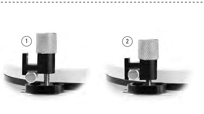
2-6 If rod height is between 1/4" [4,5mm] and 3/8" [9,5mm], use the rod clamp this way up ①. If rod height is between 3/8" [9,5mm] and 17/32" [13,5mm], use rod clamp this way up ②. Note: If the rod height is less than 1/4" [4,5mm]. See 2-7.
