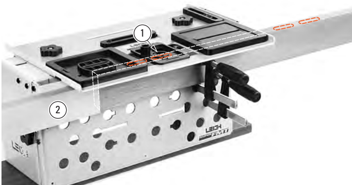
5-9 Replace the sight. Position and clamp the mortise piece so the right hand mortise of the first pair is centered under the sight ①. Either mark an outrigger or set a stop block for successive mortise pieces ②. Remove the sight and rout the right hand mortise.
