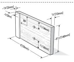
**9-4** Make the block with its side stop out of  $\frac{1}{2}$ "[13mm] stock as shown. Bore two  $\frac{1}{4}$ "[6mm] holes, countersunk for a flat head screw (part no. 287) to allow the blocks to be used at either end of the jig.
