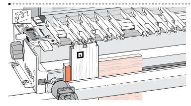
**9-3** Use the same block with side stop when cutting the tails to ensure correct alignment of the pin and tail boards.
