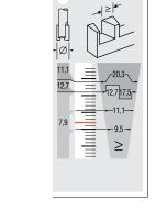
**9-6** For boards up to ½"[6mm] thick use dovetail bit 50-8 and pin bit 140-8 with the e7 or a ½6"[11,1mm] guidebush. To cut pins matching the sockets made with bit 50-8, begin with the setting shown here. Cut test pins in scrap stock and test for fit. Adjust as necessary.
