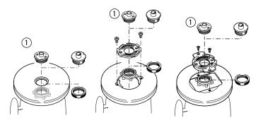
**7-1** Fit the e7-Bush ①. One is included with your D4R Pro. If the eBush is incompatible with your router, any 7/16"[11,1mm] guidebush (min. barrel length 1/4", *see page 70*) will work for all but box joints on the D4R Pro.
