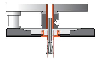
**7-6** Ideally, the router collet (and bit) should be concentric (centered) to the guidebush as in figure 7-5. Regrettably, this is often not the case; the bit can be off center (eccentric to) the guidebush ①. The illustration shows the problem highly exaggerated. The good news: bit to bush alignment doesn't affect joint fit or flushness; both are "adjusted out" in normal jig setup.
