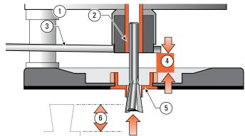
**7-2** When fitting a bit to the router ①, fit the shank as far into the collet ② as possible. Always rout with the collet as close to the guidebush as possible. Usually you can't securely grip the collet nut with a wrench ③ if the collet is at its optimum low position. Fit the bit so that the remaining travel ④ between collet and guidebush ⑤ will let the bit reach the required depth of cut ⑥.
