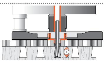
**7-3** Tighten the collet ② securely and lower the collet to adjust the depth of cut ⑥, but make sure the collet does not contact the guidebush ⑤. Some smaller collets can go down into the inside of the guide bush. Take advantage of this.
