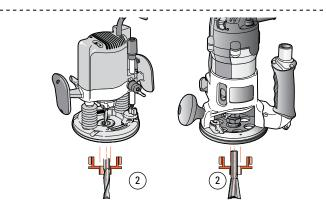
**7-7** Concentricity problems can only arise if two routers are used for through dovetails, (one for pins; one for tails). Routers with different bit to guidebush offsets 2 (misalignment shown highly exaggerated)...
