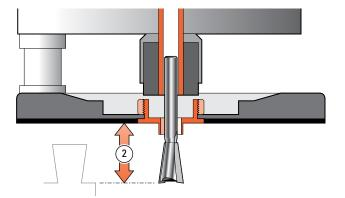
**7-5** Depth of cut is **not** the distance the bit projects from the router base. This is **bit projection** ②. This guide generally refers to depth of cut. Bit projection ③ is always .450"[11,5mm] more than depth of cut.
