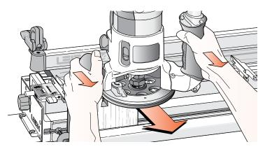
**5-6** If you insist on removing the router from the jig while it is still revolving, always pull it straight off the jig horizontally, and do not raise or lower the router until it is completely clear of the jig. With the Leigh VRS fitted to your jig you can simply park your router to one side.
