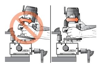
**5-5** Do not tilt the router on the jig. Keep the router flat on the jig assembly. Note: The optional Leigh VRS attachment prevents router tilting. See page vi.
