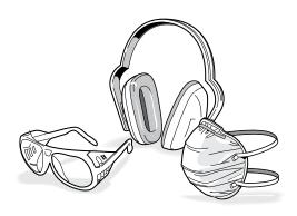
**5-2** Always wear approved safety glasses. Always wear hearing protection. Protect yourself from harmful dust with a face mask. For complete dust and waste collection, add a Leigh VRS (Vacuum & Router Support) to your jig. See page vi.
