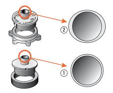
**3-2** The Leigh e7-Bush that comes with your D4R Pro is a unique template guidebush that is adjustable in size. Unlike regular circular template guidebushes ①, the e7-Bush is slightly elliptical in cross section ②. This simple innovation effectively changes the guidebush "active diameter size" when it's rotated, and provides benefits not possible with a standard round guidebush.
