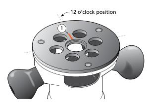
**3-5** Establish the orientation in which you normally hold and operate the router on the jig. Now, up-end the router in the same orientation. Make a small scratch line or permanent ink mark ① on the router base or eBush adaptor at the 12 o'clock position. Learn about eBush adaptors on page 69.
