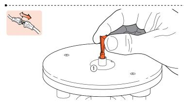
**3-7** The bit goes through the e7-Bush ① and fits in the router collet or chuck.
