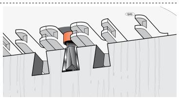
**3-8** The projecting part of the guidebush runs along the side edge of the guide finger. The rotating bit cuts the wood only, and touches neither the guidebush nor the guide surface. ■
