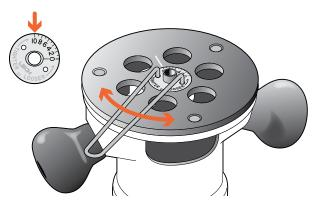
**3-6** Fit the e7-Bush to the router and align No.10 to the scratch mark. This setting is used for all through and variably spaced halfblind dovetails on the D4R Pro. Settings for single pass half-blinds, box joints and sliding dovetails are described in applicable chapters. Be sure to retighten the eBush nut after each adjustment is made with the included pin wrench.
