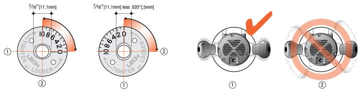
**3-3** The e7-Bush (7/16") fits the router base or a guide bush adaptor in the base (*see Appendix I*). The ellipse/oval shape has a major axis ① 7/16"[11,1mm], and minor axis ② 7/16"[11,1mm] less .020"[,5mm]. Turning the eBush 90° in the router base changes the active diameter by .020"[,5mm] providing minute adjustment and recordable settings for perfectly fitting box joints.
