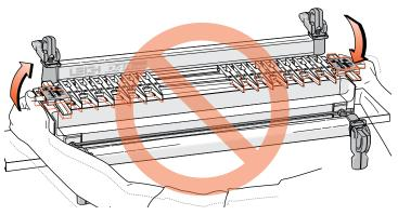
2-2 Do Not raise or lower one end of the finger assembly at a
