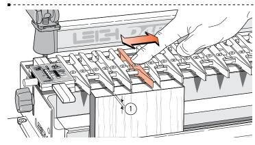
**2-3** To practice adjusting the guide fingers, put a board in the front clamp. Always raise the finger assembly slightly, approximately ½"[2mm] above the spacer board and/or workpiece ①. This is essential to allow the guide fingers to move freely on the guide finger bar and ensures that the fingers will be level and flush when locked up. Move the guide fingers by pushing on the middle to slide them along the guide finger bar.
