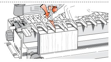
**2-4** Loosen about half the guide fingers and practice unlocking, moving, positioning and re-locking them. Always press down lightly on the center of each guide finger ① when tightening the screws.
