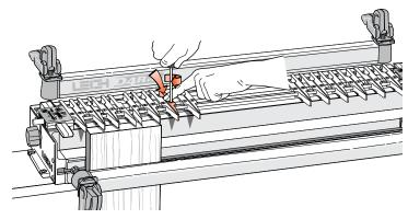
**2-6** Always tighten unused guide fingers before routing, as router vibration will cause loose screws and wedge nuts to fall out and be lost.
