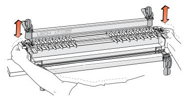
**2-1** Practice adjusting the finger assembly height. Loosen the support bracket knobs and hold them firmly. Raise and lower the assembly evenly, keeping it level, and tighten the knobs to lock it at various heights.
