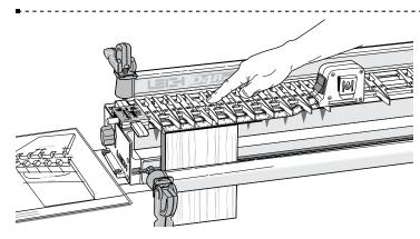
**2-7** You can adjust the guide fingers by eye, or by measurement to suit a set of plans.
