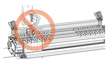
**2-5** Do not over-tighten the guide finger locking screws. The Leigh screwdriver provided will give ample torque for easy lock-up without strain.
