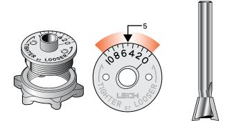
**16-4** Turn the e7-Bush to "5" and use the No. 120-8, ½"x 14° bit for sliding dovetails. This e7-Bush setting will allow for fine fit adjustment of the tail later.
