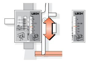
**16-18** The HB TAILS scale is not designed specifically for this mode, but it does allow you to make precise adjustments for tail size and tightness of fit on sliding dovetails.
