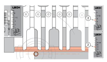
**16-13** If you use a larger guidebush, for example  $\frac{5}{8}$ "[15,9mm] rather than  $\frac{7}{16}$ "[11,1mm], move the scale in by the difference of the two guidebush radii.
