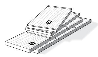
**16-26** When the fit is satisfactory, rout one end of a project tail board and test again. If the fit is good, rout all the other ends. *Note: Variations in board thickness, guidebush diameter, bit depth, angle, diameter and concentricity, make it impractical to record sliding tail size settings.*
