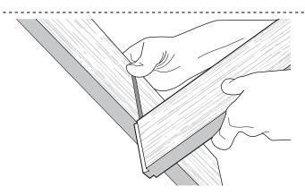
**16-23** Test the joint for fit. The tail should be too big. If it is too small, adjust the finger assembly outward by at least half the difference and rout another test tail on the other end of this test board.
