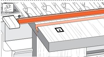
**16-16** Now rout sliding dovetail slots in the two main slot boards with the boards in the horizontal position in the rear clamp, slot side, that is inside face  $\Box$  up.
