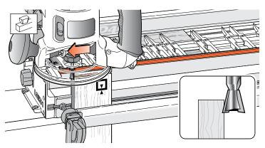
Rout one side of the test tail board.
