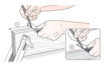
**16-7** Marking Out: *Do not mark slot positions on board faces*; mark the edges ① of both slot boards together for perfectly level shelves. Mark the narrow test slot board in the same way at several closely spaced random spots ②. This board is used only for setup.
