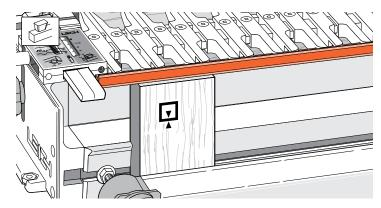
**16-17** Replace the spacer board in the rear clamp, and with the finger assembly on the spacer board, mount a test tail board vertically in the front clamp, **flush under the guidefingers**. Either side can face out  $\Box$ .
