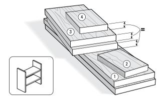
**16-6** Use  $\frac{3}{4}$ "x  $5\frac{1}{2}$ " [20x140mm] softwood to make two slot boards ①, plus one narrow test slot board ②, two tail boards ③ and one narrow test tail board ④. The tail boards ③ and test tail board ④ must be exactly the same thickness. This will make two uprights and two shelves.
