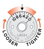
**16-25** Note: the e7-Bush fit adjustment for sliding dovetails works reverse to normal. Fit adjustments are made by adjusting the tail size only, not the socket. The e7-Bush is turned down to a lower number for a tighter fit, and up to a higher number for a looser fit. Each increment changes the glue line fit by 0.001"[0,025mm] When the fit is satisfactory, rout one end of a project tail board and test again. If the fit is good, rout all tail board ends.
