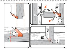
**16-5** On a full width joint, *the slot depth-of-cut should be no more than* \$\frac{1}{3}\$ the board thickness ①. If the tail board is a load-bearing horizontal member (e.g., bookshelf or step), make the tail fairly thick for good tail neck strength ②. Shorter sliding dovetails for less structural demand may be slightly deeper, with narrower profiles, especially if appearance is important ③ (e.g., where narrow rails join wider boards).
