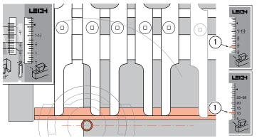
**16-12** With the finger assembly (including the sliding dovetail fence) on the support brackets in the HB TAILS mode, set the scale to 7/16"[11mm] ①. *Make sure the finger assembly is level and sitting flush on top of the board.* The HB TAILS scale was not designed for this operation, but with this setting the routed slot will be close to centered on the slot line.
