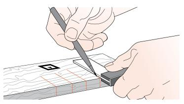
**16-8** On the test slot board only, square the marks across the face.
