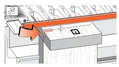
**16-14** Adjust the bit so the cut depth is about  $\frac{5}{16}$  [8mm]. Rout from left to right maintaining light inward pressure of the guidebush on the fence. Rout in only about 1"[25mm] and back out again.
