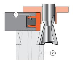
**16-19** Adjust and set the finger assembly ① so it is clear that the routed tail ② will be too large for the slot.
