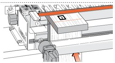
**16-10** Mount a <sup>3</sup>/<sub>4</sub>" [20mm] thick ① (yes, the <sup>3</sup>/<sub>4</sub>" [20mm] thickness is important) square-ended board vertically in the front clamp against the side stop, with the top edge butting the underside of the test board.
