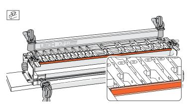
**16-1** With the finger assembly in HB TAILS mode, the sliding dovetail fence fits into the recesses in the ends of the tail guides for routing sliding dovetails.
