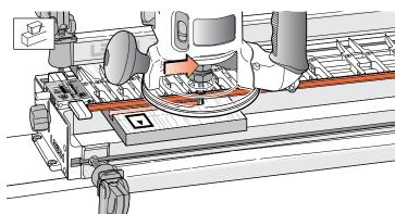
**16-2** Using the sliding dovetail fence as a guide surface for the guidebush, you can make lateral router cuts across the faces of horizontal boards (we call these dovetail *slots*), and...
