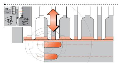
**16-15** Check to see if this short slot is centered on the pencil line. If not, adjust the finger assembly in or out and retest on the other lines as necessary until the slot is centered. Lock the finger assembly in this position and record the setting for future reference.
