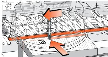
Dovetail slots preferably are routed from left to right because the bit's clockwise rotation pulls the guidebush against the fence. However; as when routing close to both ends of a board, it may be necessary to rout slots from right to left. Bit rotation will tend to pull the router away from the fence. Feed slower and maintain constant guidebush pressure against the fence.
