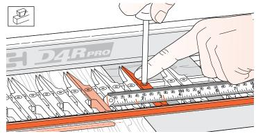
**16-28** Measure the same distance from where you want the slot stopped to a position on the finger assembly. Move a guidefinger to that point and mark the guidefinger with a felt pen as a visual router stop mark...
