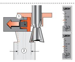
**16-24** If the tail ② is too big, move the finger assembly ① toward the jig by half the amount the tail is too big. Rout the same test board again; keep adjusting and testing until a good fit. *Use trial and error each time. It doesn't take long, and you get a good fit. For fine fit adjustment with the e-Bush see 16-25.*
