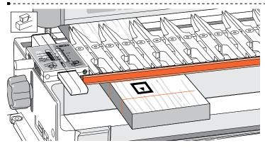
**16-9** Mount the test slot board in the rear clamp, markings up. △Dovetail slots are best routed from left to right because the bit's clockwise rotation pulls the guidebush against the fence. But when routing close to both ends of a board, you may need to rout slots from right to left. *See 16-30.*
