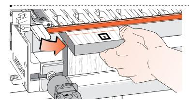
**16-11** Position and clamp the test board so that one of the edge marks is in line with the *outside edge* of the vertical board.
