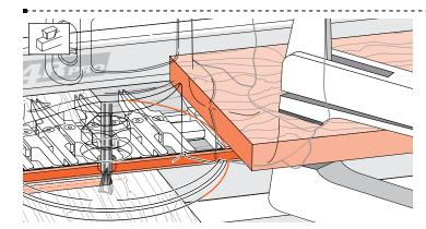
**16-29** Or lightly clamp (with a soft-jawed clamp) a short board to the finger assembly to act as a router stop.
