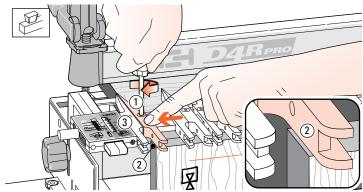
**15-4** Raise the finger assembly about ½"[3mm] to allow ease of guide finger adjustment ①. Position the second guide finger ½2"[1,0mm] in from the board edge ② and tighten the finger. The first finger stays against the scale block as a router support ③. *Note: Square ended boards are essential to achieve flush joint alignment.*
