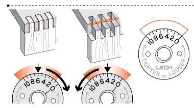
**15-11** Test the boards for fit and flushness. If the joint is loose, turn the e7-Bush to a higher number and rout two more boards. If the joint is too tight, turn the e7-Bush to a lower number. Trial-and-error establishes the best e7-Bush setting. Record it on this bush drawing for a good result the next time. *Note: each increment adjusts glue line fit by 0.002"[0,05mm]*. Retighten the eBush nut after each adjustment.
