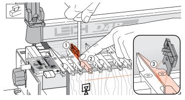
**15-6** Now place the spacer vertically on the right hand side of the third finger; the prongs to the left ①. Hold the guide finger firmly against the Spacer and tighten the second finger screw ②. As you remove the Spacer you should feel some friction ③; this indicates that the guide finger is correctly spaced.
