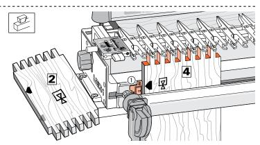
**15-16** Rout both ends of boards **2** and **4** with their edges against the Spacer and the Spacer in the No.**3** position. Keep the same edges to the Spacer.
