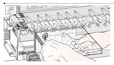
**15-3** Clamp a test board in the front left clamp, against the side stop with the top edge flush under the guide fingers. The board may be clamped face side in or out
