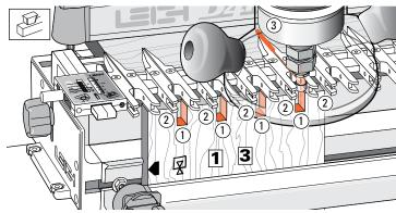
**15-20** Rout both ends of boards **1** and **3** but only rout between the guide finger openings ① not between the finger sides ②. Keep the common edge against the side stop.
