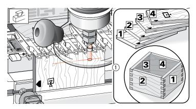
**15-19 3/4"[19mm] Box Joints** Set-up and space the guide fingers exactly as for  $\frac{3}{8}$ "[9mm] joints. Start with the same e7-Bush setting. *See 15-2 thru 15-9*.
