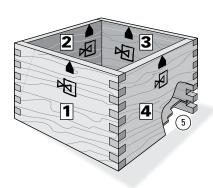
**15-17** Keeping the marked side stop edges of all boards toward the top (or all to the bottom) of the box, select the preferred outside faces before routing the grooves ⑤ for the bottom.
