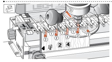
**15-21** Now rout both ends of boards **2** and **4**, with the common edge against the side stop **but only rout between the finger sides** ② not between the finger openings ①.
