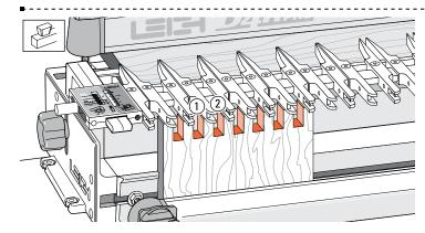
**15-9** Rout one end of the scrap board. Rout into each finger opening ① and between each finger ②. Make sure to run the guidebush on both sides of each opening.
