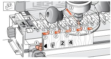
**15-22** Remove the board and fit the Spacer to the side stop with number **3** showing **4**. Now rout both ends of boards **2** and **4** again, with the common edge against the Spacer and **again** ... **only rout between the finger sides 2**, not between the finger openings **1**, steering the router mark between the pairs of finger points **3**.
