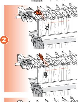
The Spacer is also used against the side stop ③ to accurately offset mating workpieces for correct board to board joint alignment.
