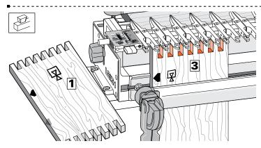
**15-15** Rout both ends of boards **1** and **3** with their **edges against the side stop**. Be sure to keep the same edge to the stop.
