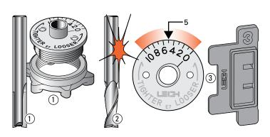
**15-1 Bit and Guidebush selection** Only the e7-Bush and the ½16" bit ① that came with the D4R Pro are required for box joints. Spiral upcut router bits ② will cut cleaner than straight flute. Where metric size bits are available an 8mm straight or spiral bit may be substituted for the ½16". Always start test routing with the e7-Bush set on "5". Note: the box joint Spacer ③ has a square notch.
