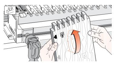
**15-14** All box joint boards are clamped alternating face side in
