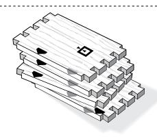
**13-4** Rout the tails on each end of the tail boards.
