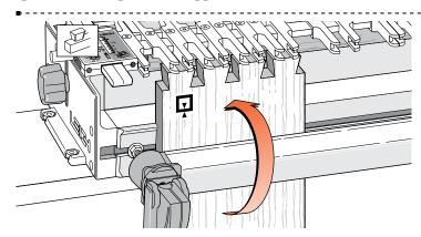
**13-3** Rout the tails. Clamp end-on-end dovetail boards in the jig for routing one end face side in and one end face side out. *Keep the same edge against the side stop for both ends.*
