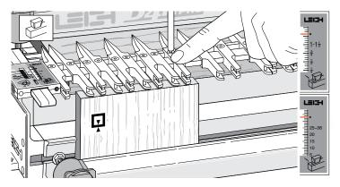
**13-2** The end-on-end dovetail is laid out in the HB TAILS mode. There is a special mark on the scale for end-on-end dovetails. Align the support bracket line with the small arrow as shown. Adjust the guidefingers as required.
