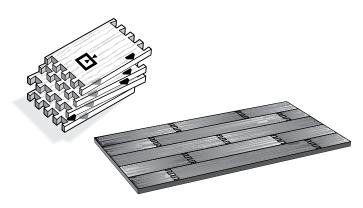
**13-6** Always assemble end-on-end joints keeping the edges of the boards that were against the side stop all in line.
