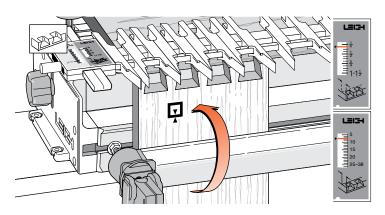
**13-5** Rotate the finger assembly to HB PINS mode and again set it on the small scale arrow for maximum pin board thickness (¾"[20mm]). There is no theoretical minimum thickness, but avoid thin board tearout, see 17-11. Rout pins on each end of pin boards, same edge against the sidestop for both ends. Narrow pins are illustrated (look like narrow tails), but guidefingers can easily adjust for even-sized tails and pins.
