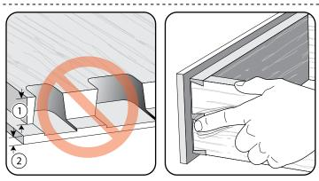
**12-8** Make sure you select a dovetail bit that has a working depth of cut less than the rabbet height ①. Otherwise, you will rout into the rabbet lip ②.
