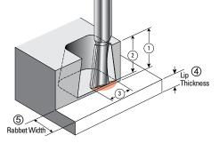
RABBET DEPTH (1) determines the maximum depth of cut (2) you can use. Select a bit with a depth of cut that is at least 1/16" [1,6mm] less than the rabbet depth.
