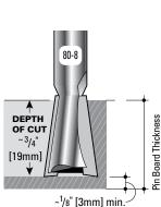
IMPORTANT: Add ~1/8" [3mm] to the depth of cut for pin board thickness NOTE: See 10-35 chart on p.38 for range of tail board thickness NOTE: Bits 80-8 and 120-8 are included with the jig ~ Symbol for approximately
