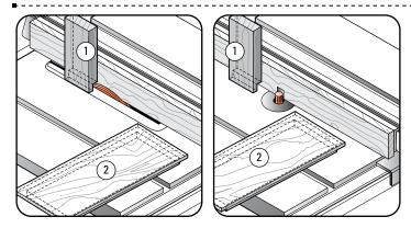
**12-5** An easy accurate way to do this is to rabbet the end of a scrap piece ① vertically over a dado blade or router bit at the same time as you rabbet the drawer front (horizontally) ②.
