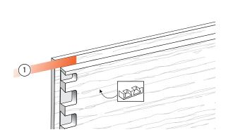
**12-7** If the rabbet width ① is greater than  $\frac{3}{8}$ "[9,5mm], the drawer side must be offset from the front side stop by the depth of the rabbet minus  $\frac{3}{8}$ "[9,5mm]. Make up a block to this measurement and stick it to the face of the jig, touching the front side stop. This will offset the drawer side away from the side stop and align the sockets with the pins.
