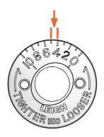
**3-7** One increment of the eBush changes the joint glue line by 0.002"[0,05mm]. Half an increment changes the fit by an incredible 0.001" [0,025mm]. A proper fit will be established with one or two test cuts.
