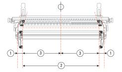
Ensure that the side stops are precisely 1½"[38mm] in from each end of the jig extrusions ①. This will position them 241/8"[613mm] apart 2 centred on the jig 3.
