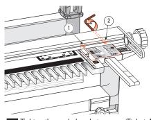
Tighten the scale bracket screws ②, but **do 5** not tighten the scale bar screws  $\mathbb{T}$  yet.
