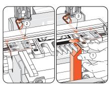
Move the combined template and bar to the Shove the complete templete and 24 left until the right side of the outer 1/4"[8mm] opening touches the block ①. Taking care to not move the template assembly, tighten the scale screws at the left end 2. Remove the block. Remove the pin and slide the template left. Tighten the scale screw at the right end ③. Your Leigh F1 is now ready for use.
