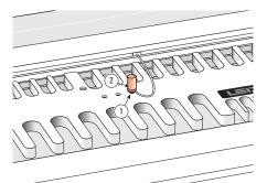
Discard the plastic shipping plug from the 6 centre hole. Align the template so that the right hand hole ① of the three central template holes aligns with the hole in the bar. Insert the template pin 2, gently twisting and pushing the tapered pin into the hole until it is fully seated.
