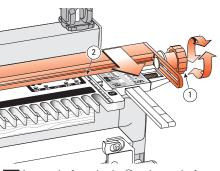
Loosen the fence knobs ① and move the fence 5 Loosen the template toward you as far forward as possible and with the fence scale reading the same at both ends 2. Then tighten the fence knobs 1.
