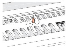
Discard the plastic shipping plug from the centre hole. Align the template so that the right hand hole ① of the three central template holes aligns with the hole in the bar. Insert the template pin 2, gently twisting and pushing the tapered pin into the hole until it is fully seated.
