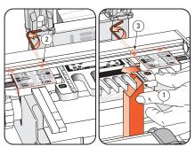
8 Move the combined template and bar to the left until the right side of the outer 1/4"[8mm] opening touches the block ①. Taking care to not move the template assembly, tighten the scale screws at the left end 2. Remove the block. Remove the pin and slide the template left. Tighten the scale screw at the right end ③. Your Leigh F1 is now ready for use.
