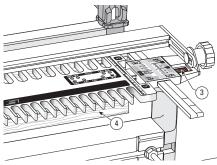
Slide the template assembly onto the jig support brackets with the  $\frac{1}{2}$  and  $\frac{1}{4}$ "[10] and 8mm] combs toward you and lower it gently onto the D4R jig's spacer board ④ (D4R UserGuide 1-1). Make sure the scale reading is the same on both scales, say on the 1"[25mm] mark, then tighten the thumb screws 3.
