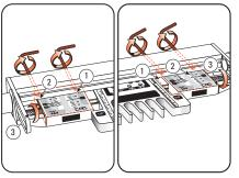
Loosen the two scale bar set screws ①, the two fence bracket screws 2, and the two scale thumb screws 3 at both ends of the template.
