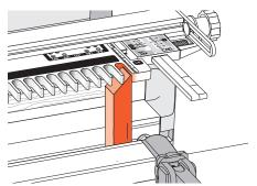
Trim off the end of a perfectly straight block at about 30 degrees. Slide the combined bar/template to allow the block to protrude into the last socket of the 1/4"[8mm] comb. Clamp the block with its vertical edge tight against the right hand side stop.
