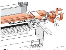
Loosen the fence knobs ① and move the fence on the template toward you as far forward as possible and with the fence scale reading the same at both ends 2. Then tighten the fence knobs 1.
