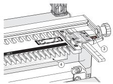
Slide the template assembly onto the jig support brackets with the  $\frac{1}{2}$  and  $\frac{1}{4}$  [10 and 8mm] combs toward you and lower it gently onto the D4 jig's spacer board ④ (D4 UserGuide 1-1). Make sure the scale reading is the same on both scales, say on the 1"[25mm] mark, then tighten the thumb screws 3.
