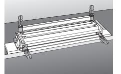
Mount the D4R jig firmly to a bench as per its instructions. Remove the dovetail finger assembly.
