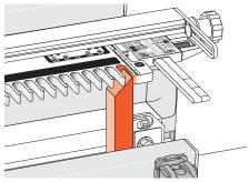
Trim off the end of an 8"[200mm) long per-Figure 1 about 30 degrees. Slide the combined bar/template to allow the block to protrude into the last socket of the 1/4"[8mm] comb. Clamp the block with its vertical edge tight against the right hand side stop.
