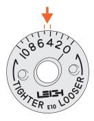
**6-7** One division of the eBush changes the joint glue line by 0.002" [0.05mm]. A perfect fit will be established with one or two test cuts.
