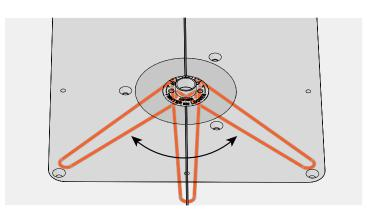
**6-6** Adjust the eBush with the pin wrench. Markings on the eBush indicate which way to turn it for a looser or tighter fit. Remember, every time you adjust the eBush you must re-tighten the eBush nut.
