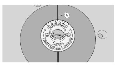
**6-5** All settings for the eBush will be aligned to the line (A) you've drawn on the router table. The line will also help guide the RTJ400.
