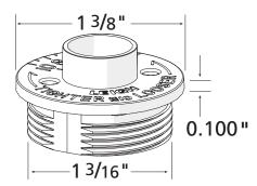
**6-3** The Leigh eBush system is designed around the decades-old Porter Cable/Black & Decker industry standard. Therefore you will likely need to adapt your router table or router table insert plate to accept a Leigh eBush with an insert ring that has a 13/8" diameter counter bore. See page 6 for details. Check with your router table or insert plate manufacturer as to what adaptation is required.
