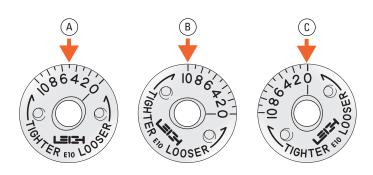
**6-2** All routing starts with the eBush in the No.5 position (a). Turning the eBush toward the No.10 position (b) results in a tighter fit because the guide bushing is now wider. Turning the eBush toward the No.0 position (c) results in a looser fit.
