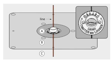
**6-4** Draw a line with a permament pen on the router table, centered on the guide bushing opening at 12 o'clock and 6 o'clock (shown in red for clarity only). This will ensure correct orientation of the eBush to the insert ring (a), the insert plate (b), and the router table (c).
