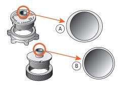
**6-1** The Leigh eBush barrel is elliptical A, unlike plain circular template guide bushings B. When rotated, the effective diameter of the barrel changes, allowing fit adjustments as small as 0.001"[0.025mm]. The e10 eBush is included with the RTJ400.
