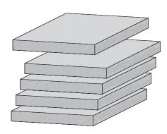
**5-1** Accurate and perfectly aligned joints require stock that is straight, flat, even thickness and equal widths, with square ends and edges. *Note: Plywood is generally unsuitable for routing because of tearout problems.*
