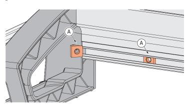
**1-3** Insert the two square nuts into the rear of the frame (A) and slide them to each end of the frame.
