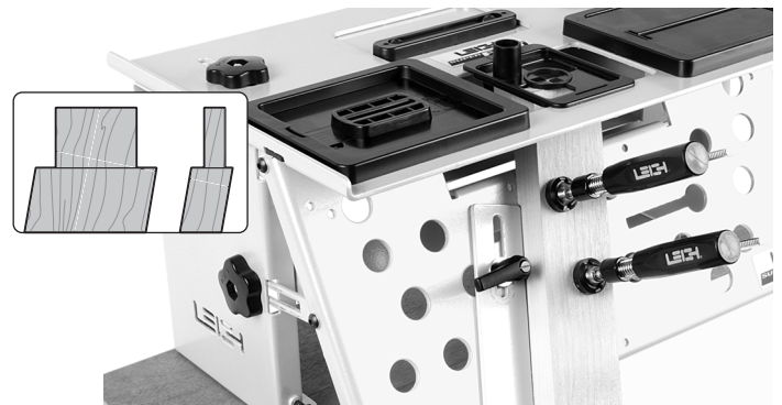
7-4 Angling both the sidestop fence and clamp plate gives a double or compound angled joint.
