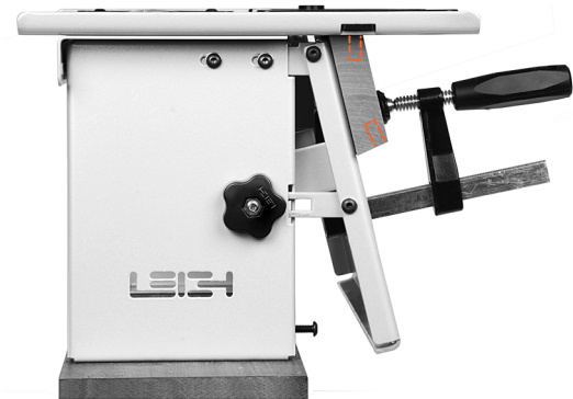
7-6 However, you may for example, want to machine spline mortises or dowel holes in a stave type construction in, say, octagons at 22½°, or hexagons at 30°, so the 30° capacity may prove to be useful. You can then machine precisely fitting splines on the Super FMT and trim them to length. ■
