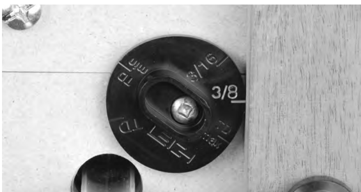
7-28 You should be thoroughly familiar with the 3/8" [9,5mm] joint procedure before routing 3/4" [19mm] joints. Set the sidestop on the 3/8" [9,5mm] mark and use the same 3/8" [9,5mm] bit and e10 eBush setting used for your successful 3/8" [9,5mm] joint fit.
