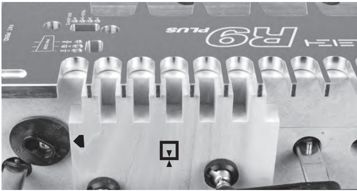
7-12 Rout all of the sockets. Remove socket board.
