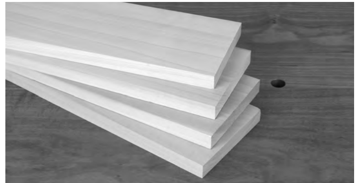
7-15 Let's make a box. Prepare four boards and mark them 1, 2, 3, and 4. Then select the grain alignment and mark the common top (or bottom) edge. Don't worry about face side selection — this can be done after routing.
