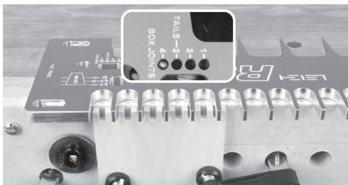
7-25 Move the template across to pin position 4 and lock. Rout all the rest of the pins.
