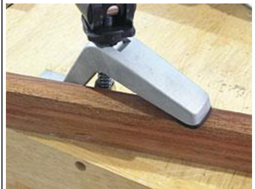
The Bench clamp in use on the workbench with clamp secured through dog holes.
