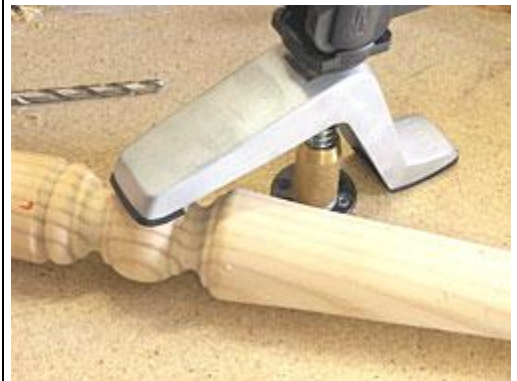
There is enough clamp force to even hold down rounded objects quite well.
