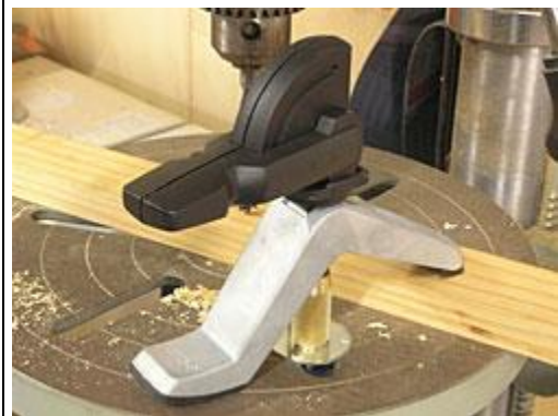
Plenty of hold-down force to secure the piece for drilling.
