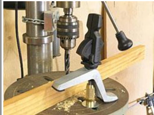
The Leigh Bench Hold Down clamp set up on the Drill Press.
