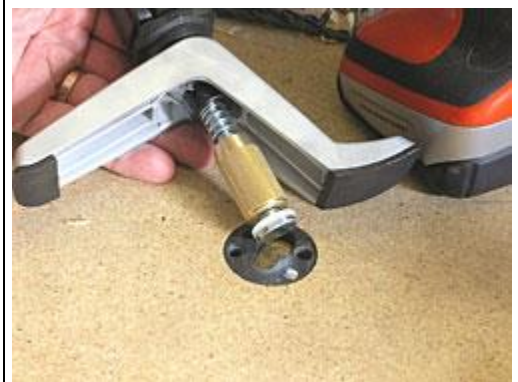
The bottom of the Surface Hold Down clamp slots into and slides in the anchor to secure the clamp to the bench.
