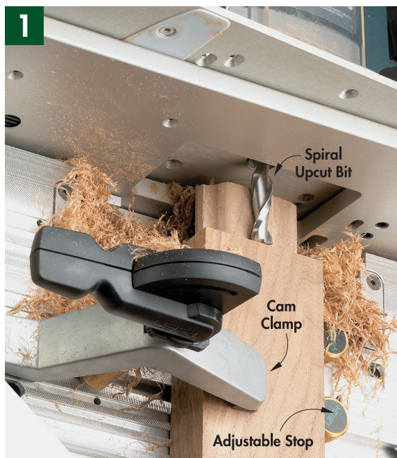
▲ Cam-action clamps and adjustable stops ensure perfect and secure placement of the workpiece. Clamps and stops can be used in various locations to accommodate different stock sizes.
