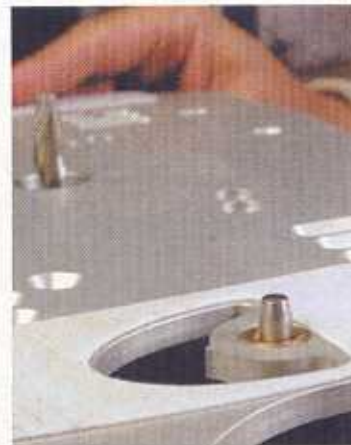
Both tapered guide pins are adjustable to allow for a tighter or looser joint
