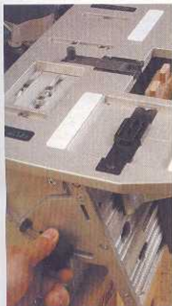
Both tapered guide pins are adjustable to allow for a tighter or looser joint
