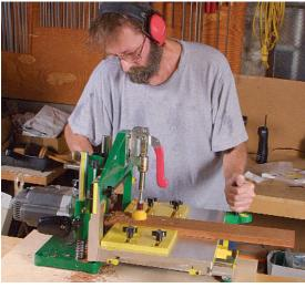
Center the workpiece on the sliding table. A toggle clamp holds the workpiece tight to the sliding table, and two yellow plastic plates bear against the edges of the workpiece to prevent any lateral movement.
