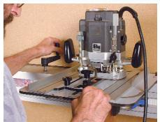
**Climb cuts are cleaner.** You can virtually solve the problem of chipout on the leading edge of the router cut by moving the workpiece in a clockwise direction around the cutter.
