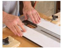
Adjust the plate to center the cut. The phenolic plate rides left to right on four loose bearings that rest on the plywood tabletop and is held in place by the two aluminum bars on both ends.
