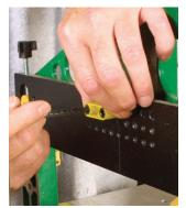
Secure a template to cut a tenon. The vellow plastic template is fastened into threaded holes in the yoke assembly with two Allen-head screws.
