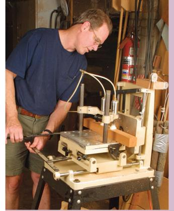
Handle controls each axis. With the Multi-Router, you have a separate handle for each of the X,Y, Z movements this machine will execute. Van Benten has used this machine in a production shop for more than 10 years, and he reports that the linear bearings on which the tables ride still work flawlessly.
