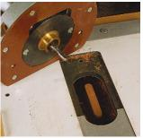
**Round or square tenons.** By varying the shape of the adjustable inserts in the phenolic plate, you can cut either round or square tenons.
