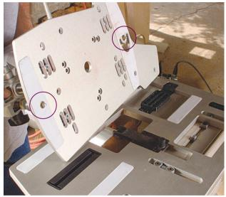
**Guidance system is finely tuned.** Visible on the left and right of the underside of the baseplate are the two tapered pins that engage grooves in the two black plastic inserts fitted into the top of the table. By changing the inserts you can cut various sizes of matching mortises and tenons.
