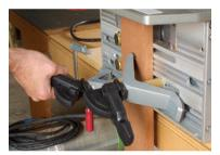
Secure the workpiece. Two cam clamps accommodate any thickness up to 3 in. and any width up to 5 in. The stock length is limited by how high the jig is mounted off the floor.
