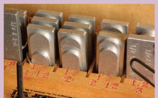
Templates guide the cut. This machine comes with 42 different templates and inserts to use with various sizes of router bits. A steel stylus on the vertical router table traces the patterns, which are mounted on the horizontal table.
