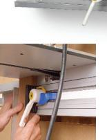
Cam clamp holds the stock in place. A cam clamp slides along a slotted track and presses the workpiece against a sturdy piece of aluminum angle.
