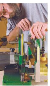
Locate the tenon cut. Vertical adjustments in the yoke assembly will affect where a tenon is cut on the workpiece. The steel stylus shown here is mounted at a fixed distance from the cutter, and you can use either the small or large end of the stylus to follow the template, which affects the size of the cut.
