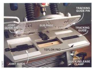
With two micro-adjust guide pins and interchangeable joint guides this jig offers great accuracy and ease of use. Several other adjustments and features, such as Teflon pads and quick-release clamps, give this tool a very focused goal—quick and accurate mortises and tenons. It's a goal at which it succeeds with flying colors.
