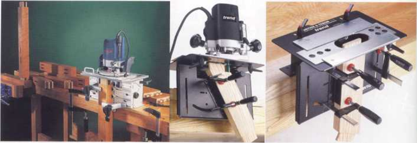
Above: Leigh's FMT jig and above centre and right: Trend Mortise and Tenon Jig
