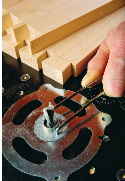
Numeric indexing on Leigh's "e10" eBush makes adjusting the fit of a joint's mating parts as easy as twisting the elliptical bushing left or right and re-routing one piece.
