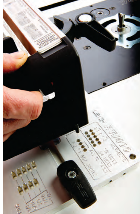
A pin under each handle enables the vertical fence to be repositioned in template holes to well-marked, automatic settings for various joint sizes and styles.
