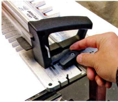
▲ The top frame locks to the comb with these latches
