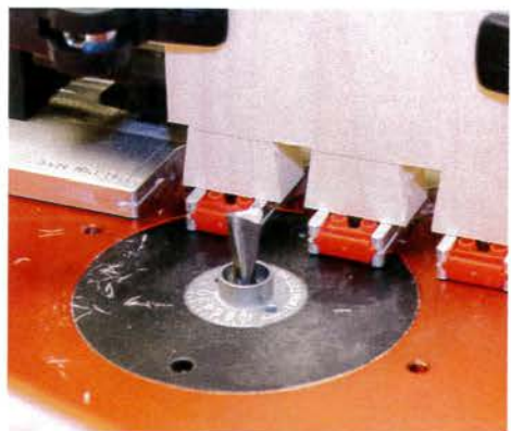
▲ The pegs prevent the guide bush from making a cut
