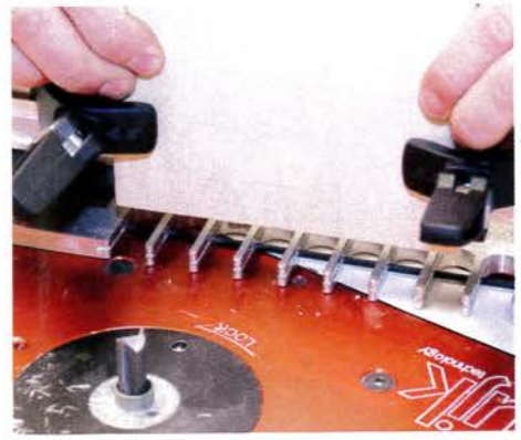
▲ It acts as a stop to limit the depth of cut on joints using thinner stock
