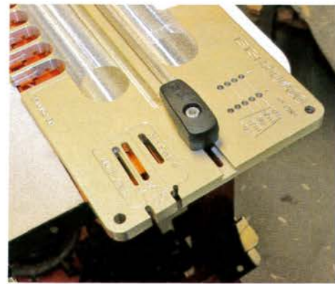
▲ Indexing shoes and slots along with etched lettering make it easy to set positions
