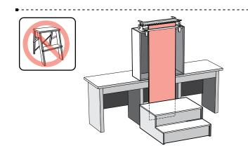
**17-15** For routing long vertical boards it may be necessary to build a jig stand to mount securely on your bench. Make the stand and bench height combination sufficient to accept the board length you have in mind. *The jig stand should be bolted securely to the bench.* Make up a stable platform to stand on as in the illustration. **Do not use a set of steps. Steps are not stable enough.**
