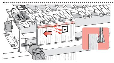
**17-13** On face cuts, whether using a straight bit or a dovetail bit, climb routing or back routing will leave a clean edge; but great caution must be exercised in controlling the router's movement from right to left, as the bit rotation pulls the router in that direction anyway
