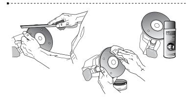
**17-21** Some router bases have sharp edges on the outside and inside corners. A slight chamfer of the edges with a fine file or sandpaper block will ease router movement on the jig. An occasional light spray of "Top Cote®" application of soft wax to the router base makes for smooth, easy router movement on the jig. ■
