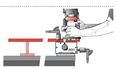
**17-16** When placing long horizontal boards in the rear clamp, make sure the rear end of the board is supported to prevent unnecessary racking of the jig.
