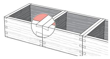
**17-18** If a number of these boxes end up side-by-side, e.g. spice caddys on a kitchen shelf, the slight misalignments of the joints could be unattractive. So when making boxes or through dovetail drawers that will be lined up beside each other with the joints showing...
