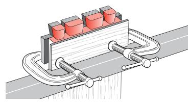
**17-12** A single scrap piece can be C-clamped on the back of halfblind tails, *but make sure you protect the workpiece from the clamp pads.* Note: There is no 100% solution to tearout. It's not the jig's fault, just something that happens when machining, sawing and even chiseling wood. Important pieces fall off from where you least want them to.
