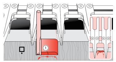
**17-1** Through Dovetail Pins With the straight bit, carefully climb-rout from right to left. Make sure you control the router firmly when climb routing.
