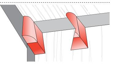
**17-8** To help prevent this, back up the cut with the end-grain of a horizontal board pushed against the back of the workpiece and held in the rear clamp. This board replaces the spacer board.
