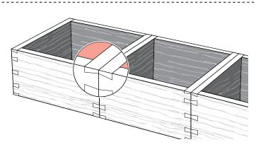
**17-19** Use the asymmetrical *mirror image* aligning techniques 14-4 to 14-11 for perfectly aligned *neighbour* joints.
