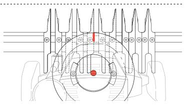
**17-20** Using The Router Mark the router base top edge at the 12 o'clock position with a felt marker pen. Without wood or bits, try some dry runs in each jig mode. This will soon get you used to positioning the guidebush against the correct guide surface without looking under the router.
