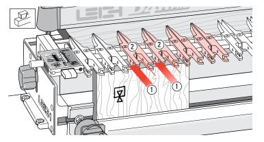
**15-7** Repeat this procedure across the jig until there is at least one guide finger spaced past the right hand side of the work piece. Finger pairs should have a uniform  $\frac{1}{2}$ "[12,7mm] space between them ①, and .054"[1,37mm] gap ② between fingers of the same pair. Tighten the unused guides.
