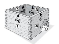
**15-17** Keeping the marked side stop edges of all boards toward the top (or all to the bottom) of the box, select the preferred outside faces before routing the grooves (5) for the bottom.
