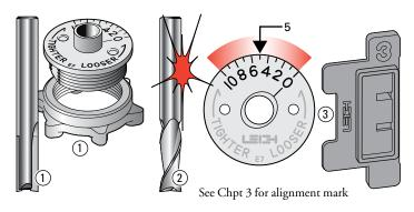
**15-1 Bit and Guidebush selection** Only the e7-Bush and the  $\frac{5}{16}$ " bit ① that came with the D4R Pro are required for box joints. Spiral upcut router bits ② will cut cleaner than straight flute. Where metric size bits are available an 8mm straight or spiral bit may be substituted for the  $\frac{5}{16}$ ". Always start test routing with the e7-Bush set on "5". *Note: the box joint Spacer* ③ *has a square notch.*
