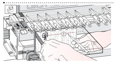
**15-3** Clamp a test board in the front left clamp, against the side stop with the top edge flush under the guide fingers. The board may be clamped face side in or out **P**. Mark and adjust the depth of cut to suit the thickness of the mating boards ①.
