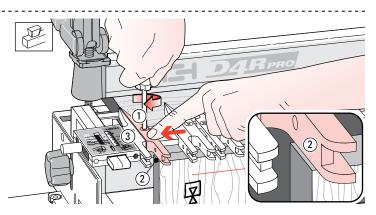
**15-4** Raise the finger assembly about  $\frac{1}{8}$ "[3mm] to allow ease of guide finger adjustment ①. Position the second guide finger  $\frac{1}{32}$ "[1,0mm] in from the board edge ② and tighten the finger. The first finger stays against the scale block as a router support ③. *Note: Square ended boards are essential to achieve flush joint alignment.*
