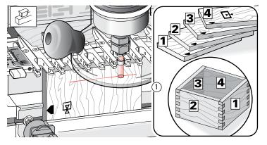
**15-19 3/4"[19mm] Box Joints** Set-up and space the guide fingers exactly as for 3/8"[9mm] joints. Start with the same e7-Bush setting. *See 15-2 thru 15-9.*
