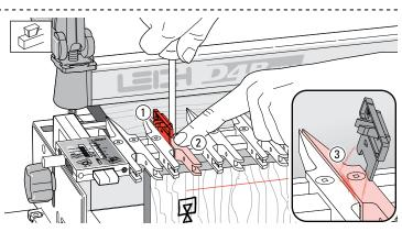
**15-6** Now place the spacer vertically on the right hand side of the third finger; the prongs to the left ①. Hold the guide finger firmly against the Spacer and tighten the second finger screw ②. As you remove the Spacer you should feel some friction ③; this indicates that the guide finger is correctly spaced.
