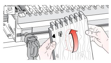
**15-14** All box joint boards are clamped alternating face side in  $\square$  and face side out  $\square$  always with the same side edge against the side stop (or Spacer).
