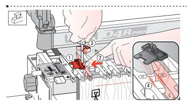
**15-5** Place the Spacer on the finger bar to the right of the second finger, numeral **1** on top overlapping the locked finger ①. Move the next finger in to touch the Spacer ②. Hold the guide finger firmly against the Spacer and tighten the second finger screw ③. As you remove the Spacer you should feel some friction; this indicates that the guide finger is correctly spaced ④.
