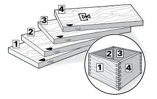
**15-13** Lets make a box with <sup>3</sup>/8" box joints.. Prepare four boards and number them **1** to **4**. Then select the grain alignment and mark the common top (or bottom) edge **▶**. Don't worry about face side selection; this can be done after routing.
