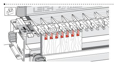
**15-9** Rout one end of the scrap board. Rout into each finger opening ① and between each finger ②. Make sure to run the guidebush on both sides of each opening.
