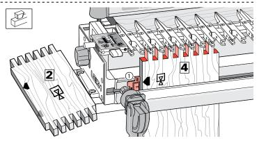
**15-16** Rout both ends of boards **2** and **4** with their **edges against the Spacer**. Have the Spacer in the No.**3** position ①. Keep the same edges to the Spacer.
