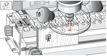
**15-8** Lower the finger assembly onto the spacer board and doublecheck that the bit depth is down to the center of the pencil line ①. Make sure the collet does not rub on the guidebush.
