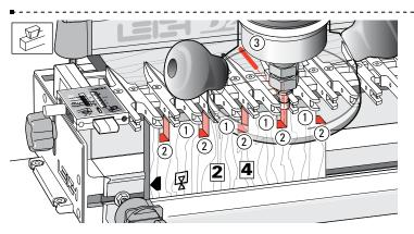
**15-21** Now rout both ends of boards **2** and **4**, with the common edge against the side stop **but only rout between the finger sides** (2) not between the finger openings (1).
