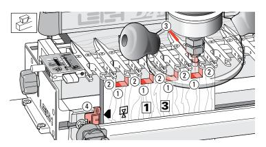
**15-23** With the Spacer still in position rout both ends of boards **1** and **3**, with the common edge against the Spacer and **only rout** between the finger openings ①, steering the router mark along the finger points ③.
