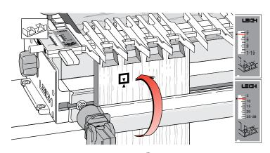
**13-5** Rotate the finger assembly to HB PINS mode and again set it on the small scale arrow for maximum pin board thickness (¾"[20mm]). There is no theoretical minimum thickness, but avoid thin board tearout, see 17-11. Rout pins on each end of pin boards, same edge against the sidestop for both ends. Narrow pins are illustrated (look like narrow tails), but guidefingers can easily adjust for even-sized tails and pins.
