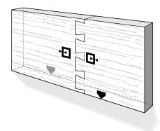
**13-1** End-on-end dovetails are made in the same modes as half-blind joints, but both boards are routed vertically in the front clamp, alternately face side in and then face side out  $\square$ . Boards for end-on-end joints may be up to 3/4" [20mm] thick.
