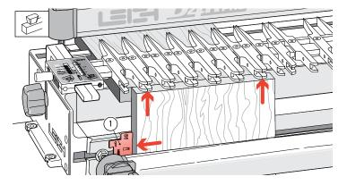
**11-15** Unclamp the tail board from the front clamp and insert the dovetail spacer as shown against the side stop ①. Re-set the drawer side in the front clamp so that its top edge touches the guide fingers and is perfectly flush with the top face of the drawer front and the left edge is against the Spacer.
