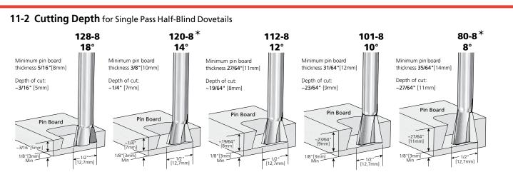
**IMPORTANT:** Add at least  $\frac{1}{8}$  [3mm] to the depth of cut for pin board thickness. **NOTE:** See 11-9 chart on p.42 for range of tail board thickness. \* Included with jig ~ Symbol for "approximately"
