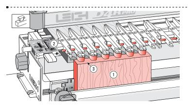
**11-25** For tail (drawer side) boards thicker than 9/16" [14,29mm] ①, set the scale to 1/2" [12,7mm] ② and leave the stop rod in place. **Do** not set the scale to the actual tail board thickness. With thicker boards, more of the inside portion of the tail board ③ will be routed away. Slight scale adjustments may be required for a flush fit. See figures 11-20 through 11-22.
