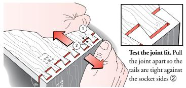
**11-18** If the joint is loose, lower the bit to increase the depth of cut by the amount of the gap at the bottom of the pins ①. If the joint is tight, raise the bit slightly to decrease the depth of cut. Test again. If there is a gap at only one end of the joint, the boards have been routed at different depths. Check the finger assembly is flat on the pin board and the tail board touches the bottom of the fingers.
