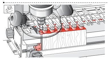
**11-17** Now rout in and out from left to right. Follow the guides in on the left of each finger opening to touch the stop rod and come out on the right. The pins, tails and sockets are formed simultaneously.
