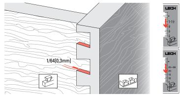
**11-22** If the tails fit in too far past the pins ends, set the HB TAILS scale **toward the operator** by half the amount required.
