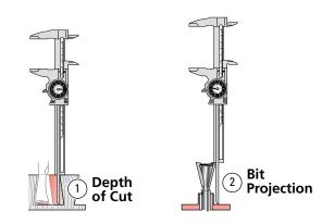
**11-4** Cumulative plus/minus tolerances in routers, bits and guidebushes, make it impossible to state exact bit depth for first-time precision fit. All dovetail jigs require trial and error tests to attain a fine fitting joint. The good news; we give a starting depth for each bit. Test and measure the successful 'Best fit' depth of cut ① or bit projection ② and record for future first-time fits.
