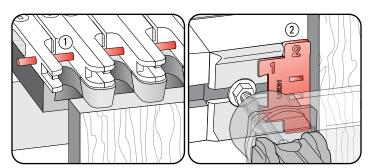
**11-7 Stop Rod & Dovetail Spacer** Insert the Stop Rod through the holes in the fingers ① to convert them from deep tail sockets to a shallow fixed comb. The flexible stop rod is fed through the holes in the fingers from the "far" end of the jig. The **Dovetail Spacer** (note the dovetail shaped notch) snaps into the channel against the left-hand front side stop ② to correctly offset the drawer sides from the drawer fronts. After setup, the Spacer stays in place for the complete procedure.
