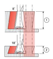
**11-3 Bit Angle and Depth of Cut** Half-blind pins and tails are routed with the same dovetail bit, the same guidebush, and the same depth of cut. A different depth of cut requires a different angled bit. Leigh offers five different angled dovetail bits for a range of cut depths. A lesser angle, say 8°, for a deeper cut ①; a greater angle, say 18°, for a shallower cut ②.
