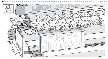
**11-11** With the scale set on ½"[12,7mm], lower the finger assembly to about ½"[3mm] above the drawer front to ease adjusting the guide fingers ①. *The scale is always set on the 1/2"[12,7mm] mark for single pass dovetails.*
