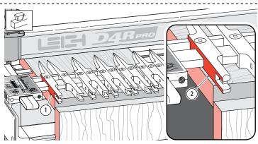
**11-12** With boards the same width as a board width chart size (Fig. 11-8), set the first guide finger flush against the board edge ① and tighten. If board width is greater than a chart size, set the first finger in from the edge by half the additional board width ②. If board width is narrower than a chart size, overhang the first finger by half the difference and tighten.
