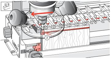
**11-16** Insert the Stop Rod through the holes in the fingers ①. Mark a line on the board that matches the depth of cut required from 11-2. *For the first light cut, move router from right to left using firm control, as it's driven in this direction by the bit.* Only the tip of the bit should cut on the first pass ②. This back, or climb routing, leaves a very clean shoulder when routing across grain.
