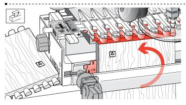
**11-23** To make a box, repeat the procedure four times, ensuring the drawer fronts, rears and sides are all rotated correctly in the jig, keeping the inside face **I** of the boards away from the jig.
