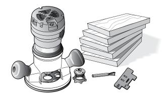
**11-5 Routing a Test Joint** You need a router, the e7-Bush set at No.10 (see chapter 3 for e-Bush instructions) and one of the bits listed in 11-2. For this example we used the 80-8 <sup>1</sup>/<sub>2</sub>"[12,7mm] 8° dovetail bit. *Note: Dovetail bits rout at a shallower depth for single pass half-blind dovetails than for regular variably spaced half-blind joints (See Chapter 10).*
