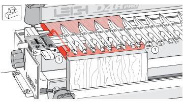
**11-10** Place a sample drawer front from  $\frac{5}{8}$ " to  $\frac{1}{2}$ " thickness [16 to 38mm] in the rear clamp. Clamp with the side edge against the left rear side stop, front end edge touching flush across the rear of the front board ①. Note: the  $\frac{5}{8}$ " [16mm] minimum thickness can be reduced if using other shallower bit depths. ! *Board edges must be square.*
