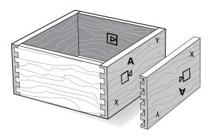
**11-24** Assemble the drawer. As with through dovetails, it doesn't matter which edge of any of the boards are at the top or bottom, the drawer will still fit together e.g. pin board "A" can be up either way.
