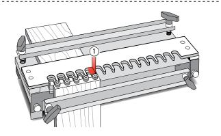
**11-6** This is a typical fixed template comb type jig. The comb depth (1) is usually dimensioned to suit the most popular drawer side thickness of  $\frac{1}{2}$ "[12,7mm].
