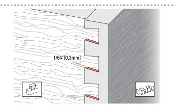
**11-19** Keep the test tail board that fits well, and mark it with the number of the bit you used to rout it. For quick set-up next time, clamp this tail board in the jig as a *depth-of-cut gauge* ① to show how far to lower the bit. Better yet, measure the bit projection from the end of the guidebush ② or guidebush flange ③ and record this for fast set-ups in future.
