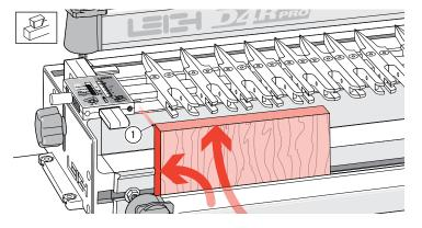
**11-9** With the finger assembly raised in the *HB* Tails mode, clamp a drawer side in the front left side, against the side stop and the top end edge slightly above the jig body top ①.
