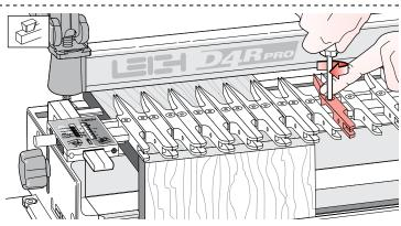
**11-14** Move any spare fingers so that they will support the router and **tighten all loose fingers**.
