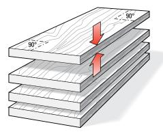
**6-1** It is vital for accurately aligned joints that stock used on the Leigh jig must be prepared straight, flat, of even thickness and equal widths, with square ends and edges. *Note that plywood is generally unsuitable for routing because of tearout problems.*
