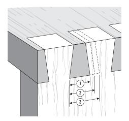
Note that some of the dovetail bits' depths of cut overlap. For example: No.70-8 bit (B) :  $\frac{1}{4}$ " -  $\frac{1}{2}$ " [6 - 13mm] No.75-8 bit (B) :  $\frac{3}{8}$ " -  $\frac{5}{8}$ " [9,5 - 16mm] No.80-8 bit (B) :  $\frac{1}{2}$ " -  $\frac{13}{16}$ " [12 - 20mm]
