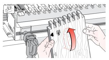
**15-14** All box joint boards are clamped alternating face side in ☐ and face side out ☐ always with the same side edge against the side stop (or Spacer).
