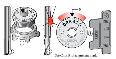
**15-1 Bit and Guidebush selection** Only the e7-Bush and the 5/16" bit ① that came with the D4R Pro are required for box joints. Spiral upcut router bits ② will cut cleaner than straight flute. Where metric size bits are available an 8mm straight or spiral bit may be substituted for the 5/16". Always start test routing with the e7-Bush set on "5". *Note: the box joint Spacer* ③ *has a square notch.*
