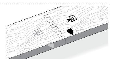
**15-18** The same method will produce end-on-end joints.
