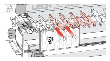
**15-7** Repeat this procedure across the jig until there is at least one guide finger spaced past the right hand side of the work piece. Finger pairs should have a uniform ½"[12,7mm] space between them ①, and .054"[1,37mm] gap ② between fingers of the same pair. Tighten the unused guides.
