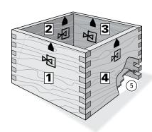
**15-17** Keeping the marked side stop edges of all boards toward the top (or all to the bottom) of the box, select the preferred outside faces before routing the grooves ⑤ for the bottom.
