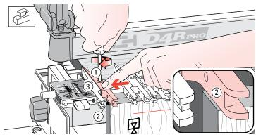
**15-4** Raise the finger assembly about  $\frac{1}{8}$ "[3mm] to allow ease of guide finger adjustment ①. Position the second guide finger  $\frac{1}{32}$ "[1,0mm] in from the board edge ② and tighten the finger. The first finger stays against the scale block as a router support ③. *Note: Square ended boards are essential to achieve flush joint alignment.*
