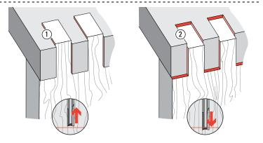
**15-12** If the joint is over flush ①, raise the bit slightly. If it is under flush ②, lower the bit.
