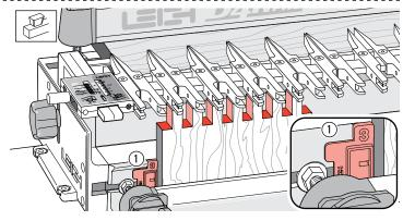
**15-10** Remove the board and fit the box joint Spacer against the front side stop with the **number 3 showing** ①. Make sure it is fully home. Clamp the second test board with its side edge against the Spacer and its top edge touching the guide fingers. Rout this board. *Note: Square ended boards are essential to achieve flush joint alignment.*
