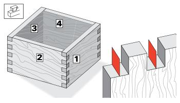
**15-24 Joint fit** Check for joint fit as usual, and repeat testing if required. Theoretically, there will be nothing in the <sup>3</sup>⁄<sub>4</sub>"[19mm] sockets, literally a zero thickness wall, where the bit has passed by twice. However, routing tolerances can leave a very thin "wall" uncleared by routing. This can be quickly removed with a chisel or sandpaper. ■
