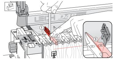
**15-6** Now place the spacer vertically on the right hand side of the third finger; the prongs to the left 1. Hold the guide finger firmly against the Spacer and tighten the second finger screw 2. As you remove the Spacer you should feel some friction 3; this indicates that the guide finger is correctly spaced.
