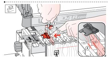
**15-5** Place the Spacer on the finger bar to the right of the second finger, numeral **1** on top overlapping the locked finger ①. Move the next finger in to touch the Spacer ②. Hold the guide finger firmly against the Spacer and tighten the second finger screw ③. As you remove the Spacer you should feel some friction; this indicates that the guide finger is correctly spaced ④.
