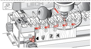
**15-22** Remove the board and fit the Spacer to the side stop with number **3** showing **4**. Now rout both ends of boards **2** and **4** again, with the common edge against the Spacer and **again** ... **only rout between the finger sides 2**, not between the finger openings **1**, steering the router mark between the pairs of finger points **3**.
