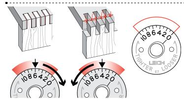
**15-11** Test the boards for fit and flushness. If the joint is loose, turn the e7-Bush to a higher number and rout two more boards. If the joint is too tight, turn the e7-Bush to a lower number. Trial-and-error establishes the best e7-Bush setting. Record it on this bush drawing for a good result the next time. *Note: each increment adjusts glue line fit by 0.002"[0,05mm]*. Retighten the eBush nut after each adjustment.
