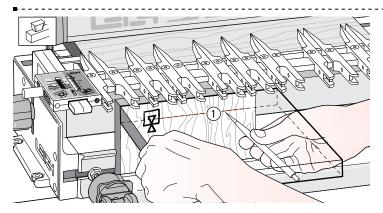
**15-3** Clamp a test board in the front left clamp, against the side stop with the top edge flush under the guide fingers. The board may be clamped face side in or out
