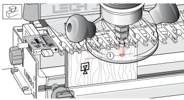
**15-8** Lower the finger assembly onto the spacer board and double-check that the bit depth is down to the center of the pencil line ①. Make sure the collet does not rub on the guidebush.
