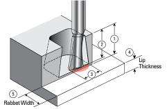
**RABBET DEPTH** ① determines the maximum depth of cut ② you can use. Select a bit with a depth of cut at least 1/16'' [1,6mm] less than the rabbet depth.
