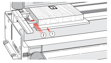
**12-3** Provided the drawer front lip is  $\frac{3}{8}$ "[9,5mm] or less in thickness ①, you can mount and rout rabbeted drawer fronts **and sides** exactly the same way as flush drawer fronts. If the lip is thicker or wider than  $\frac{3}{8}$ "[9,5mm] ② *see 12-6 thru 12-8.*
