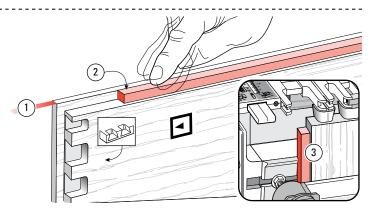
**12-6** If the lip thickness ① is greater than <sup>3</sup>/<sub>8</sub>" [9,5mm], it will not fit under the side stop. Block the drawer side away from the front side stop by exactly rabbet depth (*see 12-3*). Make up a block ② and stick it to the jig face ③ with double-sided tape. Make sure it touches the side stop. This will offset the drawer side from the side stop by the width of the rabbet, and align the sockets with the pins.
