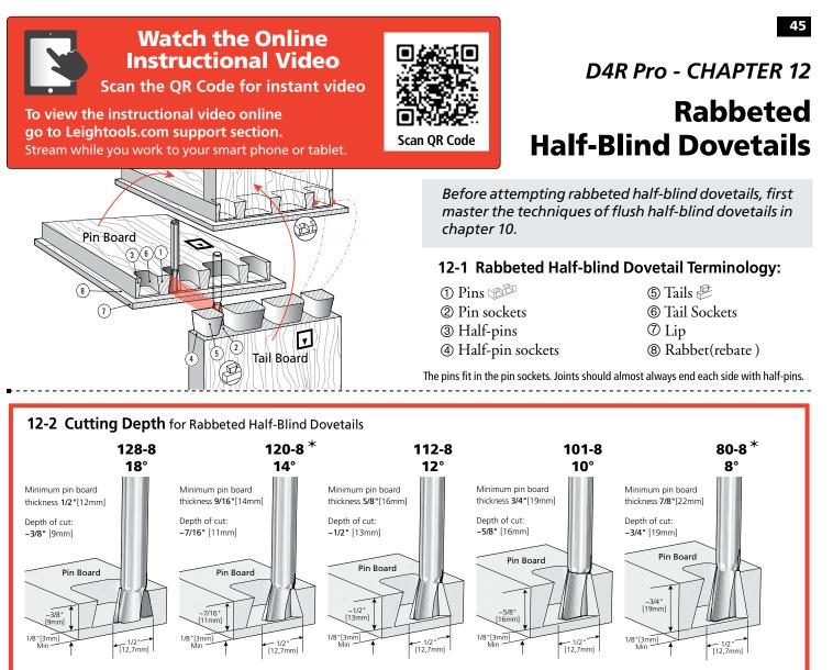
**IMPORTANT:** Add at least  $\frac{1}{8}$  [3mm] to the depth of cut for pin board thickness. **NOTE:** See 10 - 35 chart on p.38 for range of tail board thickness.  $\star$  Included with jig ~ Symbol for "approximately"
