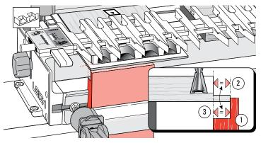
**12-4 Rabbeted Pins** You will need to clamp a scrap stop block ① in the front of the jig out from the jig's front face by exactly the depth of the rabbet ②. This brings the pin ends exactly in line with the front jig face ③, ensuring that the scale reading is accurate.
