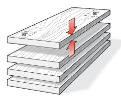
**6-1** It is vital for accurately aligned joints that stock used on the Leigh jig must be prepared straight, flat, of even thickness and equal widths, with square ends and edges. *Note that plywood is generally unsuitable for routing because of tearout problems.*
