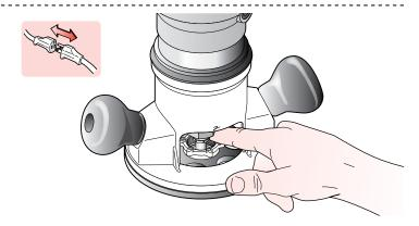
**5-4** Always disconnect the power source from the router when fitting bits or guidebushes, or making adjustments. Before connecting the router to the power source, make sure the
