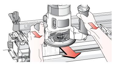
**5-6** If you insist on removing the router from the jig while it is still revolving, always pull it straight off the jig horizontally, and do not raise or lower the router until it is completely clear of the jig. With the Leigh VRS fitted to your jig you can simply park your router to one side.
