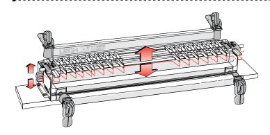
**4-3** The finger assembly is raised or lowered using the support brackets to suit different thicknesses of horizontal boards. ■
