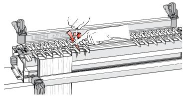
**2-6** Always tighten unused guide fingers before routing, as router vibration will cause loose screws and wedge nuts to fall out and be lost.
