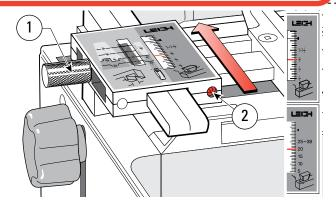
Slide the complete finger assembly with loose scales onto the support brackets. Set the bracket index line at ¾ "[20mm] on the # HB TAILS scale and tighten the thumbscrews ①. Tighten the scale screws ② firmly with the hex key provided. If the scales are removed from the finger bar for any reason, follow this procedure to re-attach them.
