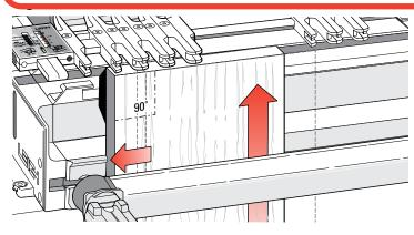
**1-11** You will operate the cam-action speed-clamps every time you use the jig, so get used to the feel of the clamps first. Use some square ended boards for practice. Make sure the end of the board is touching the underside of the guidefingers. Then slide the board over against the side stop.
