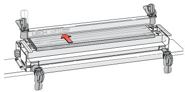
**1-19** For all but the wider workpieces, you need only operate the clamp on the workpiece end ① of the jig to release the board. For narrower boards, the clamp at the free end ② should be just tight enough to bow the clamp bar about 1/8"[3mm] 3 greatly exaggerated in this view.
