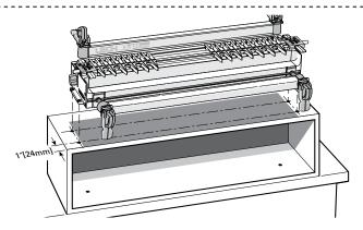
**1-22** To gain height for a more comfortable working position or for routing longer boards, mount the jig to a box that can be bolted securely to a bench.
