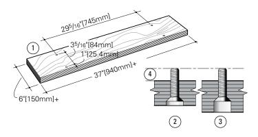
**1-1** Prepare a flat mounting board (MDF or Plywood), 3/4"[20mm] thick and min. 37"x 6"[940x150mm]. Drill (4) 9/32"[7mm] holes on 29 5/16"x 3 5/16"[745x84,2mm] centers, 1"[25,4mm] in from front edge of board ①. Countersink ② or counterbore underside ③ if board is thicker, so (4) 1/4-20x1" long machine screws project above the top surface by 3/8"[9,5mm] ④.
