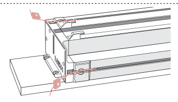
**1-3** With the jig right side up, insert one square nut (part #284) into each of the channels in the main extrusion. These nuts are for possible future attachment of accessories. *See Chapter 9.*
