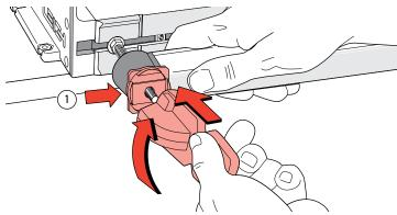
**1-6** Place one black step washer ① on each T-bolt with the *flat side against the clamp bar*. Screw a clamp lever assembly onto each T-bolt, **making sure the cam lobes are between the step washer sidewalls**.
