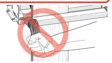
**1-12** Do Not force the cam-action speed-clamp. It has great leverage, and excessive force may damage the workpiece or the
