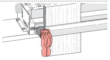
1-18 Then adjust the clamp until the clamp lever is in the right position at the right pressure.
