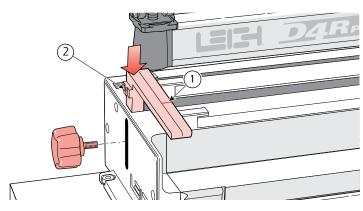
1-7 Insert the finger assembly support brackets. Note: The right and left support brackets are NOT interchangeable. Ensure the raised lug @ faces outwards when the bracket is installed. For clarity, the set line ① is drawn in red. The actual lines are black.
