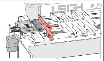
Loosen the thumbscrews and make sure the finger assembly slides on and off the support brackets smoothly, in both the tail and pin modes. Move the outermost guidefinger at each end of the finger assembly outward to touch the scales, and tighten. If fingers do not slide easily, see note on page 7. This finger acts as an end support for the router and is not generally used as a guide.
