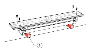
**1-2** Turn the jig body upside-down on two blocks ① (to protect the side stops). Using the four nuts and four countersunk machine screws, bolt the base board to the jig using the two nut recesses in each end housing. Holes drilled 1"[24mm] from the front edge of the board go to the front of the jig. Now you can clamp your D4R to any bench.
