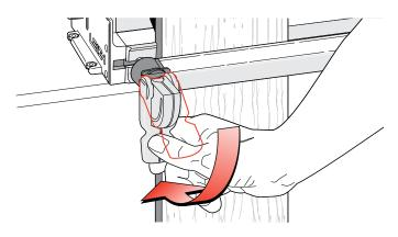
1-13 A smooth, firm action is enough to engage the clamp. Rule of thumb: If you can't throw the lever comfortably by pressing the end of it with your thumb, reduce the tension. A few minutes of trial and error will help you feel the right clamp tension. Firm thumb pressure is about right.
