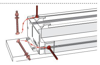
**1-4** Insert the four clamp T-bolts into the T-slots (two at each end of the jig). Position so that the washers seat into the round milled recesses. Tighten the four clamp bolt nuts with the Leigh wrench.
