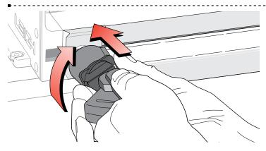
Release the clamp, remove the board and turn the step washer a quarter turn (the step height inside the step washer is one quarter of the thread pitch).
