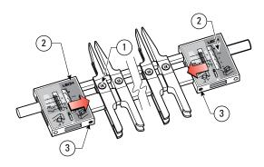
Place the finger assembly on your bench with the guidefinger screws ① on top and the pointed ends of the guidefingers away from you. Fit the scales onto the finger assembly, placing the # HB TAILS scale @ to the right at both ends. Do not tighten the scale set screws 3 yet. Note: The 1/4" square half-blind pin bar is supposed to be shorter than the finger bar. It is not inteneded to fit in the scales at both ends.
