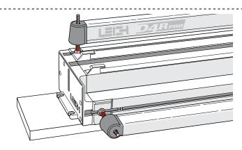
**1-5** Place four springs and two clamp bars on the T-bolts. Make sure the clamp bars move freely on the T-bolts.
