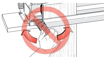
**1-14** Do Not use the lever as a torque arm. Adjust the clamp tension only with the clamp disengaged.
