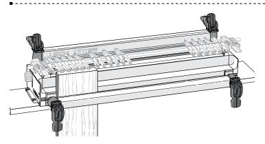
**1-15** When engaged, the front clamp levers should point down and the rear clamp levers should point away from the operator.
