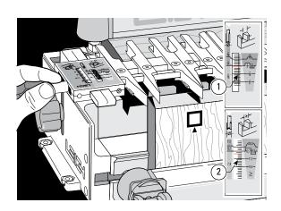
Where finger assembly scales overlay an illustration, the "inches" scale ① will be at the top, and "millimeters" scale ② at the bottom. Only the right hand "active" half of the scales are illustrated. For clarity, setting positions are indicated with a red line in the guide only. On the jig, the lines are black.
